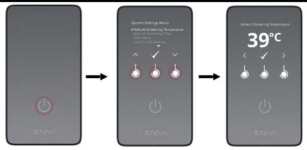
Touch and hold the Start/Stop icon (¹) for five seconds whilst ENVi® is in Standby to enter the System Settings. Touch the circular symbols under the Up ∧ and Down ∨ chevrons to browse System Settings Menu, and use the circular symbol under the tick ✓ to select the option.
