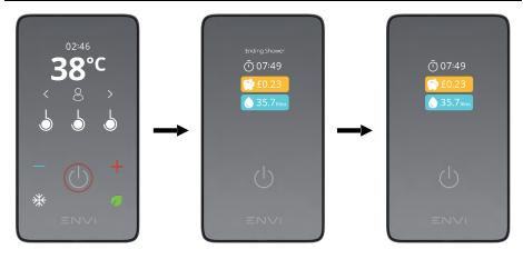
Once the timer has elapsed, or if the **Start/Stop icon** () is touched whilst showering, ENVi® will enter phased shut down, which protects the Tri-HUB by purging it of hot water before turning fully off.
