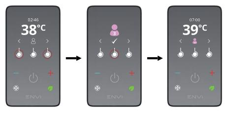
Touch the circular symbols under the left  $\langle$  and right  $\rangle$  chevrons to browse and the circular symbol under the tick  $\checkmark$  to select between six User Profiles. Upon selecting a User Profile, the shower will automatically adjust the shower temperature and timer to the personalised settings.
