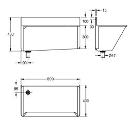
Surgeons scrub up trough manufactured from 1.5 mm thick,grade 304 stainless steel, with a satin polish finish. supplied with 38mm waste outlet in the base of the trough for surface mounting. The top and bottom areas of the trough are fixed to the wall using joggle strips. Wall fixing screws and plugs are not supplied. L or R after the code number refers to the handing of the waste outlet ie. left or right when facing the front of the trough. Rear waste outlet version also available.
